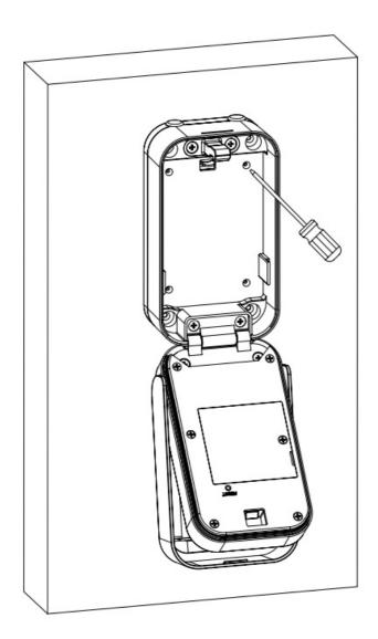
3. Drill hole & install wall plugs Drilling depth: (D6x40mm)
