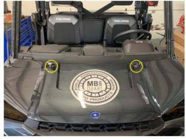
• Remove two push pins from the center cup holder
