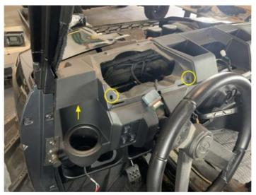
• Connect harness and place the instrument panel in location and then insert two push pins
