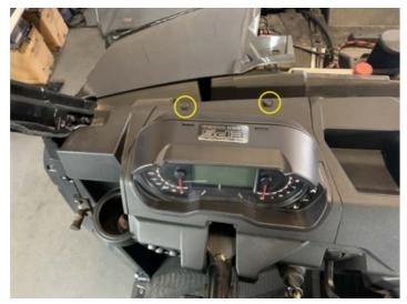
• Install three push pins on passenger side dash
