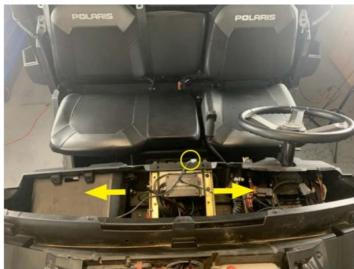
• Reaching from the top of the driver's side of the dash, pass the white wires through the top of the pocket and insert the grommet
