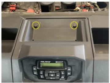
• Remove two push pins from the instrument cluster. Remove and disconnect the connector on the back
