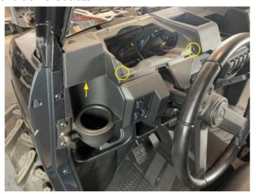
• Remove six push pins from the front of the dash
