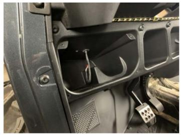
• Reaching from the top of the passenger side of the dash, pass the gray wires through the top of the pocket and insert the grommet
