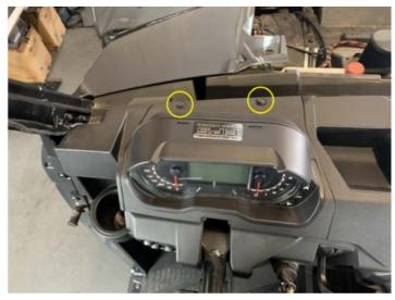
• Open the upper glove box and remove four T20 Torx screws and then lift the assembly out of the vehicle
