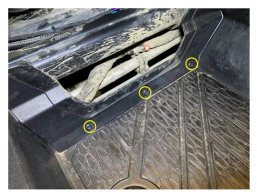
• Install passenger grab handle with four 13mm bolts
