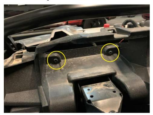
• Carefully pull dash toward rear of vehicle by door opening on driver and passenger sides
