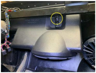
• Tighten three M5 bolts on top of enclosure with a 4mm allen wrench and also tighten two T40 Torx bolts and three Phillips self tapping screws on the front of the plate
