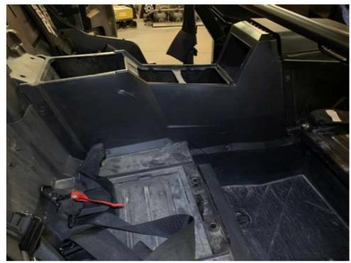
• Install rear glove box in rear center console (Remember to connect wires to bottom 12-volt accessory port)
