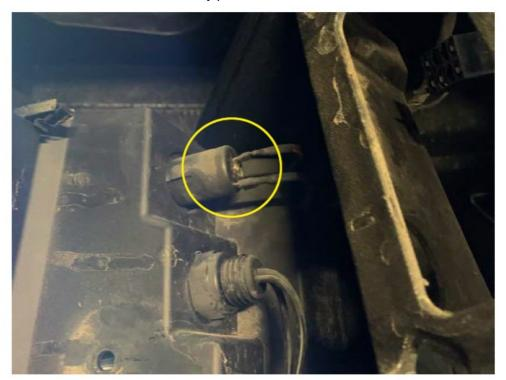
• • Remove plastic nut from ignition switch and remove from dash
