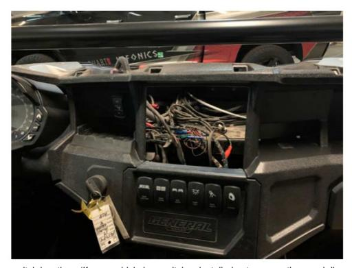
• Remove lower switch locations (If your vehicle has switches installed note connections and disconnect)
