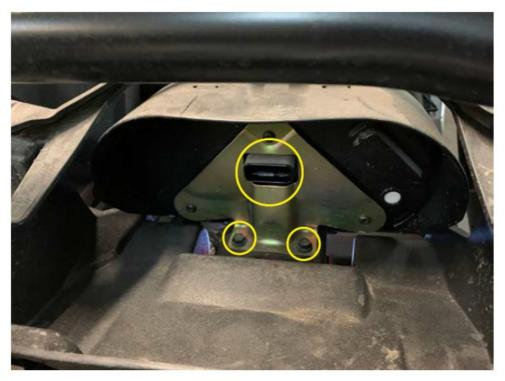
• Disconnect the connectors from the back of the light and four wheel drive switches
