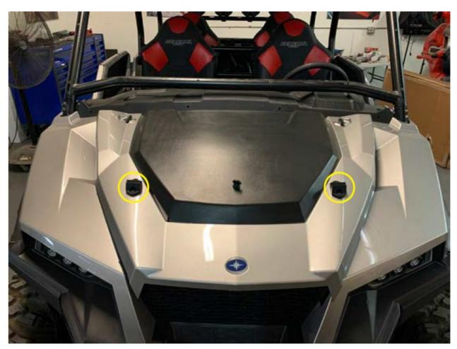
• Remove seven push clips from front of dash
