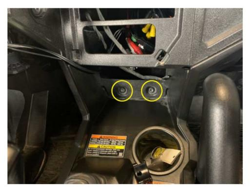
• Install two T40 bolts in passenger glove box
