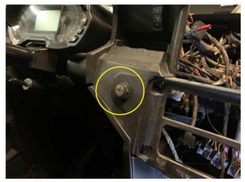
• Lower the steering column and disconnect wiring from the back of the instrument cluster and emove the two 10mm bolts to remove the instrument cluster
