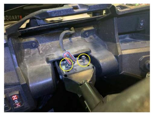
• Install two T40 bolts in center console
