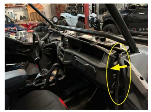
• Carefully remove dash from vehicle by lifting up and out of the vehicle
