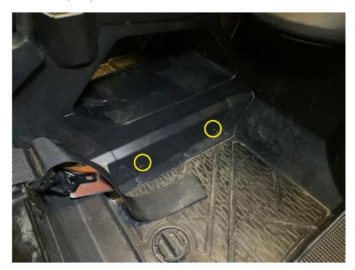
• If two-seat skip ahead if four-seat, then install rear console and install six push pins on driver and passenger side
