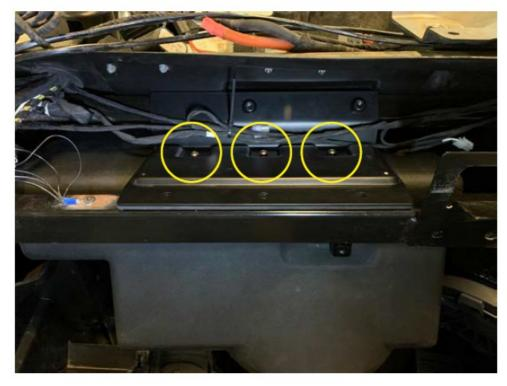
• Rotate enclosure toward bracket lifting upward and using a 4mm allen wrench, loosely install the three M5 button head bolts with thread patch to the top of the enclosure
