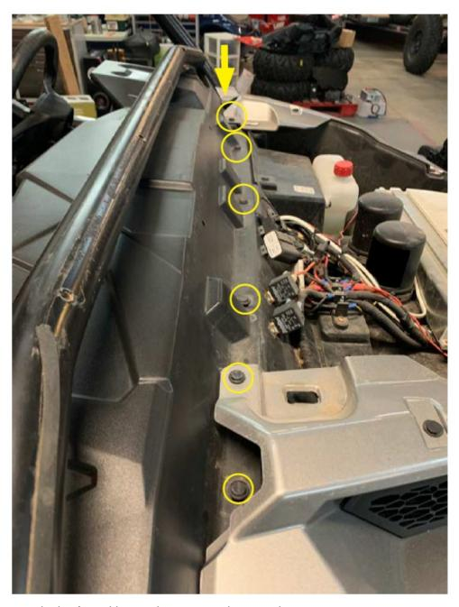
• Remove top two push pins from driver and passenger door opening
