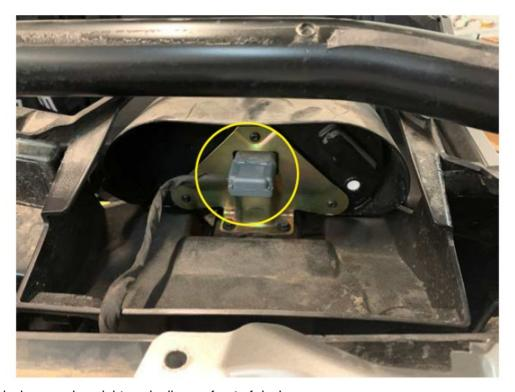
• Install top of dash, snapping eight push clips on front of dash
