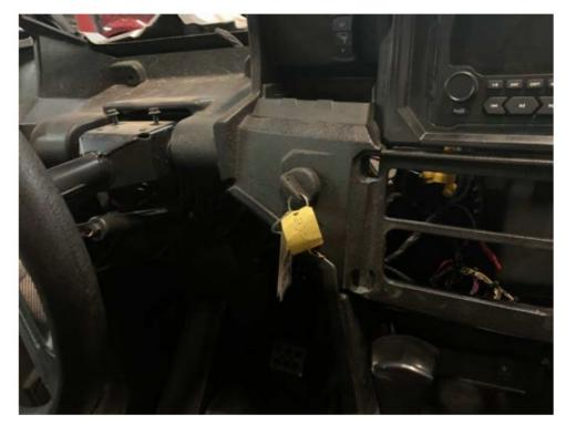
• • Install two T40 bolts on driver side instrument cluster area
