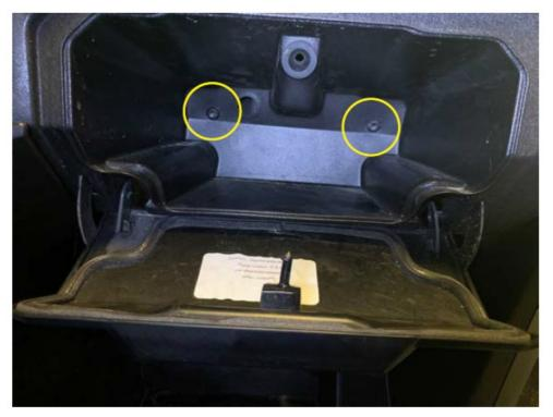
• Install instrument cluster with two 10mm bolts
