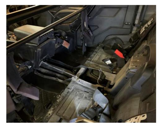
• Remove two push pins from lower front center console and remove
