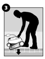
3. Put the Pool Cleaner into the pool. Release the Pool Cleaner and let it sink to the floor of the pool. Make sure that the floating cable is free of any obstructions.
