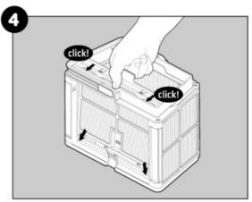
Assemble the filter panels.
