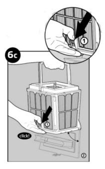
• Open the latch to release the bottom lid in order to remove the debris.
