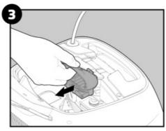
3. Pull the impeller cover backwards torelease it. Clean the debris trapped around the impeller. Assemble the impeller cover.
