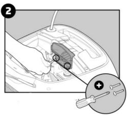
2. Using a short screwdriver open the 2 screws.
