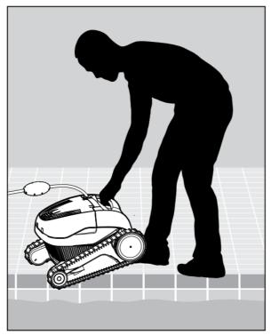
5.2.1 Put the Pool Cleaner into the pool. Release the Pool Cleaner and let it sink to the floor of the pool. Make sure that the floating cable is free of any obstructions.
