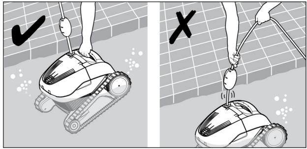
5.3.2 Using the floating cable, bring the Pool Cleaner to the pool's edge. Using the handle, remove the Pool Cleaner from the pool.
