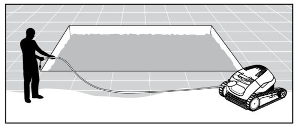
5.1.2 Unwind the cable and stretch it out completely so that it has no kinks.
