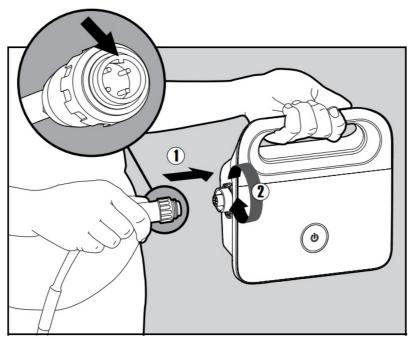
5.1.3 Attach the floating cable to the power supply by inserting it with the notch on the connector (1), lined up with the groove in the socket on the power supply, and turning clockwise (2).
