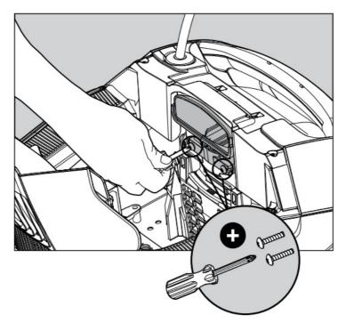
8.1.2 Using a short screwdriver open the 2 screws.
