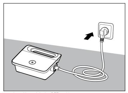
5.1.4 Plug in the power supply and leave it in the OFF position.
