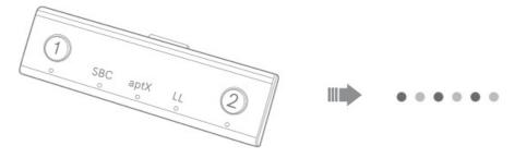
4. Pairing is successful when the LED on the PodsKit changes from flashing white to constant white.
