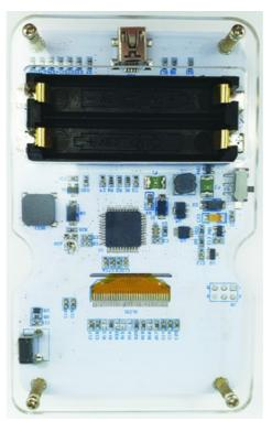
**Please Note:** The holes of acrylic bottom board should be aligned with the potentiometer on the console when installing it.
