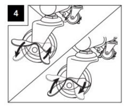
A4: Turn the wings of the brake to apply or release it.
