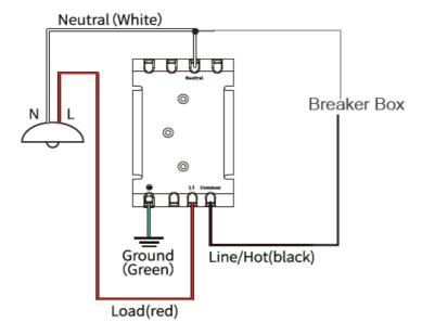
Cap oft the remaining Li Wire (RED) from the Switch with a Wire nut. Wire the Smart Dimmer 3-Way
