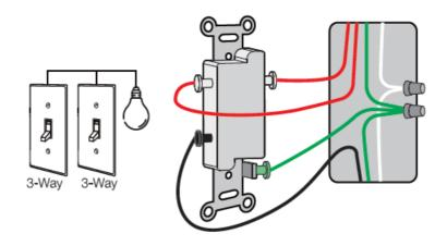
Identify Line, Load, and Neutral Wires
