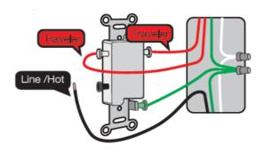
Neutral wire is required to install the smart dimmer .Most likely a bundle of one or more white wires in the wall. GROUND wires are usually BARE COPPER or GREEN.
