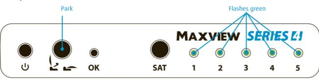
**PARK** – Press and hold for 3 seconds. LED's 1 to 5 flash green to indicate system is collapsing. Once fully collapsed, control panel can be powered off.
