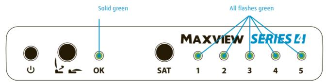
• C. Ignition mode parking. When the antenna is parking using the Ignition (green wire) all sat LEDs flash green.
