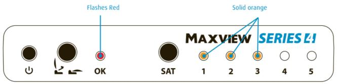
• **F.** Elevation Error. If elevation motor stops the above LED sequence will occur, please contact Customer Services.
