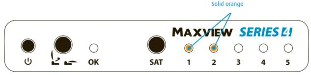
• E. Azimuth Error. If rotation motor stops the above LED sequence will occur, please contact Customer Services.
