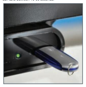
4. When the SYNC LED goes out turn off the Control Box power and remove the USB flash memory stick.
