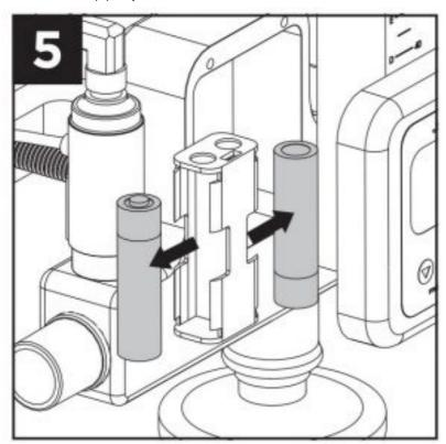
6. Ensure correct orientation and install two (2) new batteries.
