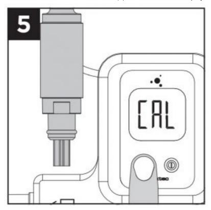
6. Insert sensor into port on MaxVenturi.
