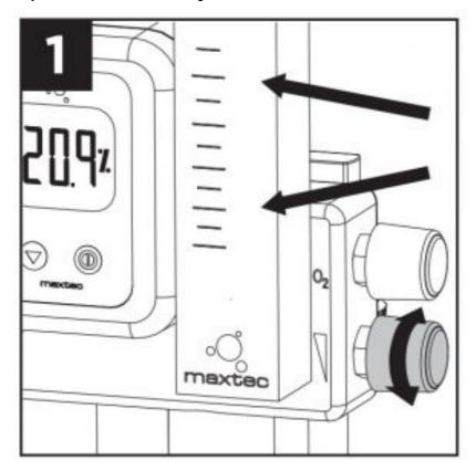
2. Set desired oxygen mixture by opening O2% knob and read analyzer.
