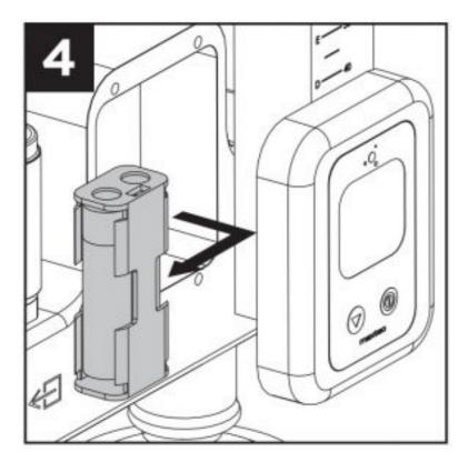
5. Remove two (2) depleted batteries.
