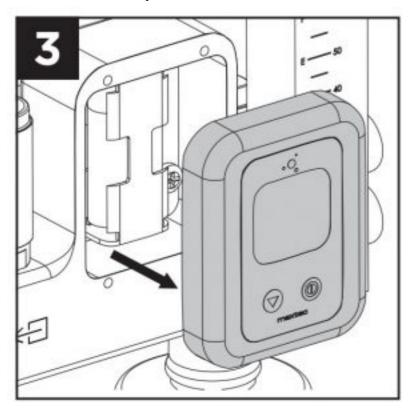
4. Remove battery pack from rear wall of cavity. Use caution with wires.
