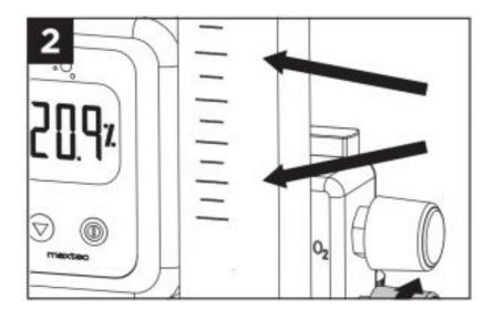
WARNING: Adjusting the oxygen setting too high at low flows may cause oxygen to exit the air inlet port. Verify the direction of flow by placing your hand under the air filter to feel for air escape
