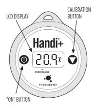
**CALIBRATION BUTTON:** Press the calibration (CAL) button to adjust the calibration value to reflect the known oxygen concentration. To simplify operation, the Handi+ Analyzer automatically determines the calibration gas being used as room air (20.9%) or high grade (100%).
