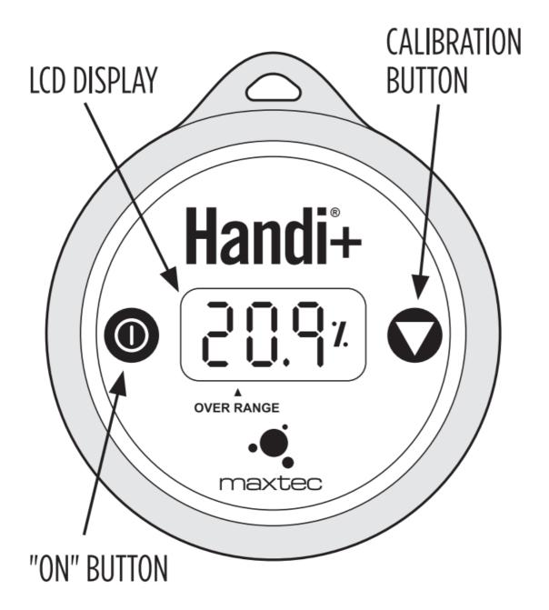
**ON/OFF BUTTON:** Use this button to turn the Handi+ on and off. When the Handi+ is in the Sleep (power off) mode, the LCD display is blank. The analyzer turns off after 1.3 minutes if no buttons are pressed.
