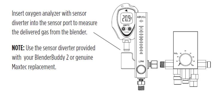
**NOTE:** A small continuous sensor bleed is provided to the analysis port which enables gas analysis regardless of which outlet port is used on the blender.
