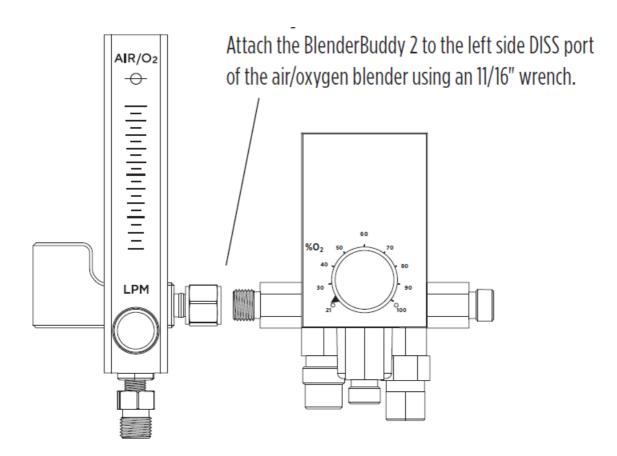
**NOTE:** Low flow BlenderBuddy 2 models (3, 15 and 30 LPM) should only be used with Low Flow blenders. High Flow BlenderBuddy 2 models (70 LPM) should only be used with High Flow blenders. Use outside these applications may result in flowmeter inaccuracies.
