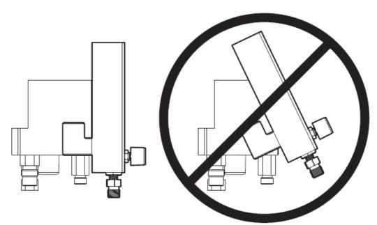
Align the flowmeter in an upright, vertical position with the blender and firmly tighten the fitting. **NOTE:** Ensure the fitting is completely tightened to prevent rotation during use.
