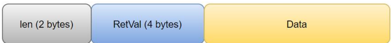
Figure 33. Adapter response for GPIO commands.
