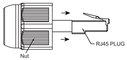
3. Split open the seal and insert the cable through the seal.
