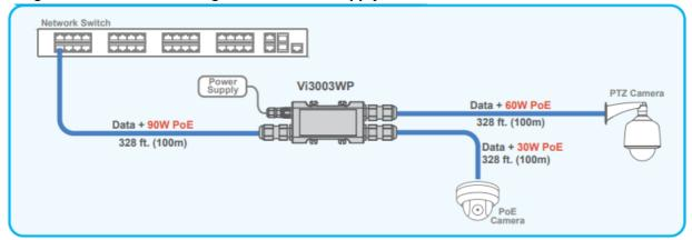
Vi3003WP allows for the transmission of two cameras over a single cable run or adding a new camera close to an existing camera.
