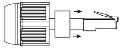
4. Insert the cable through the gasket.
