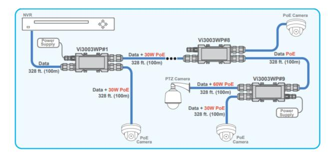
A total of 9 IP addresses can be accessed on a single cable run. eliminating the need for network switches.
