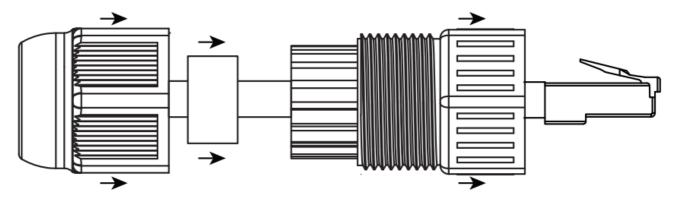
5. Tighten the nut to seal the cable.
