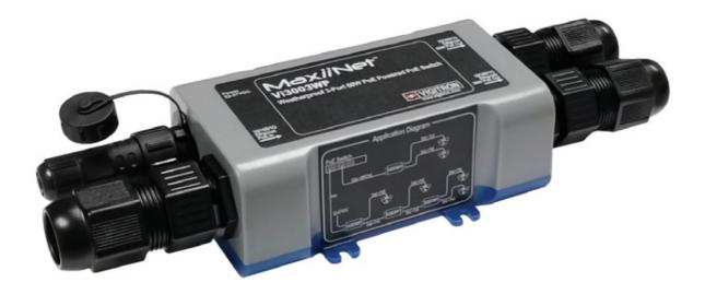
The Vi3003WP is a 3-port Layer 2 weatherproof Ethernet and PoE switch providing drop and insert capability for connecting several IP devices along a single cable run. The Vi3003WP provides a cost effective method for increasing distances beyond the standard Ethernet limit of 328 feet (100m) for 10/100/1G Mbps Ethernet. Multiple units can be cascaded to provide up to nine IP cameras to be connected to a single network switch port over distances of up 3,000 feet (909m).
