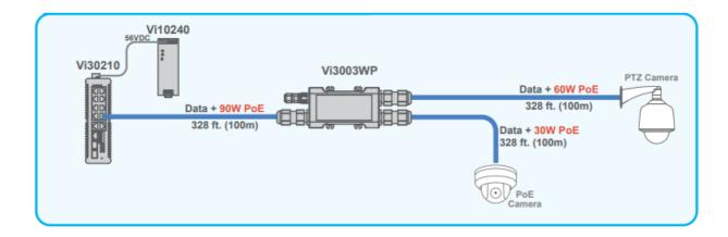
Vi3003WP allows for the transmission of two cameras over a single cable run or adding a new camera close to an existing camera. The PoE Midspan provides power to the Vi3003WP and both cameras.
