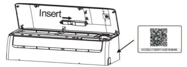
Open the front panel, unscrew the display cover and remove it, then insert the smart kit into the reserved interface(For model B). Reinstall the display cover.
