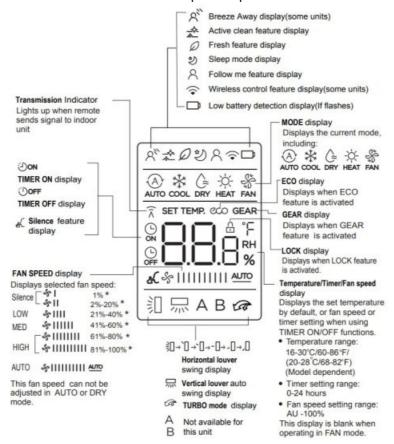
Note: [\*] Not all the models can display the fan speed values between AU-100%.
