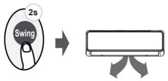
If continue to press the SWING button, five different airflow directions can be set. The louver can be move at a certain range each time you press the button. Press the button until the direction you prefer is reached.
