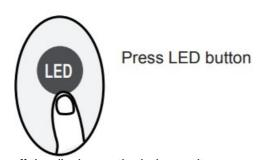
Press this button to turn on and turn off the display on the indoor unit.
