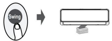
Keep pressing this button more than 2 seconds, the vertical louver swing function is activated. (Model dependent) **Airflow direction**
