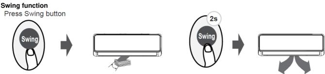
The horizontal louver will swing up and down automatically when pressing Swing button. Press again to make it stop.
