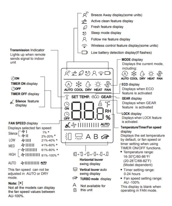
This fan speed can not be adjusted in AUTO or DRY mode.
