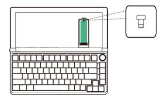
Step 3: Press the silicone clasp into the hole position, cover the hard disk cover and complete the installation.
