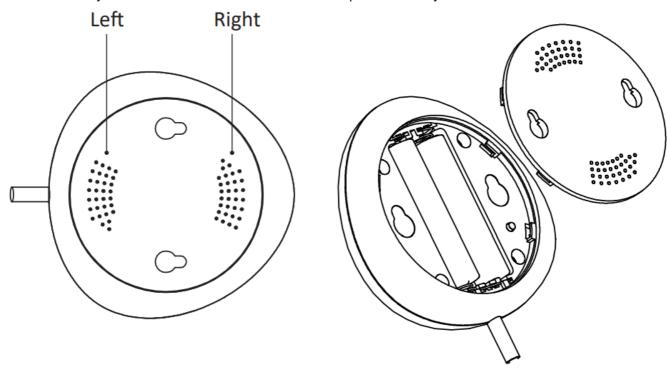
2. Put 2xAAA batteries in with the correct positive and negative electrode.
