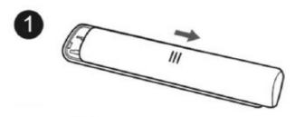
2. Insert two AAA batteries according to the polarities marked on the battery case.
