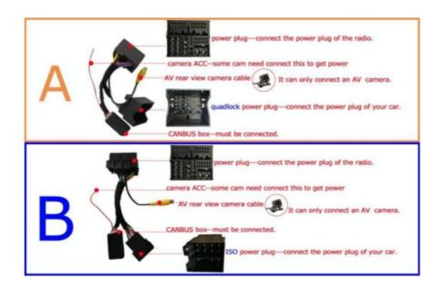
Volkswagen cars have three different power interfaces, namely PQ quadlock, ISO plug and MQB quadlock. See the diagram below:
