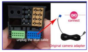
After installing the camera, please test it by closing the trunk to avoid the camera not working due to the reverse lights not functioning. If you still encounter installation issues, please refer to the instructions and contact our customer service. 99% of the problems can be resolved.
