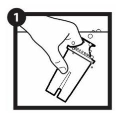
1. Place the filter into a bowl of clean cold tap water, push gently down until submerged and bubbles of air are released. Leave for 15 minutes.
