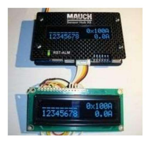
If the Hub X8 is installed in a place where the display is no more visible, then you can connect here a standard 2×16 LCD display (4-bit data bus), but please do not use any LCD displays with back LED light, as these lights can draw easily more than 200mA and the supplied power from the Power-Cube might be not enough.
