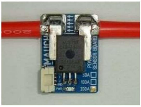
Please connect here any of PL-xxx sensors. However, all sensors must be of the same current ra $\Theta$ ng! If you use less than 8 sensors, then it doesn't matter where you connect the sensors. However, sensor 1 must be always connected, via the 4p cable for voltage measurement.
