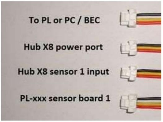
1st 4p -> To PL or PC / BEC 1st 3p -> Hub X8 power port 2nd 3p -> Hub X8 sensor 1 input 2nd 4p -> PL-xxx sensor board 1 The supply voltage is 4.95-5.05V and the max. current should not exceed 0.5A. The current draw of the Hub X8 (with active OLED) is 50mA, plus 8x 15mA (current sensors) = 170mA (0.17A) So even if we connect 2pcs X8 with 16 current sensors, plus a Hub X2 (15mA), we're still below the 0.5A. ( $2 \times 0.17A$ ) + 0.015A = 0.335A
