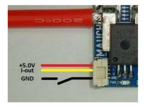
If all 8 possible sensors are installed, but you want to fly your UAV with only 4 LiPo's, then you can deactivate the unused current sensors, by either disconnecting them from the Hub X8, or installing a switch into the GND wire of the sensor board.
