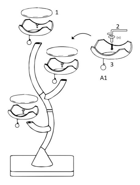
A1: Tighten the screws with tool (C).
