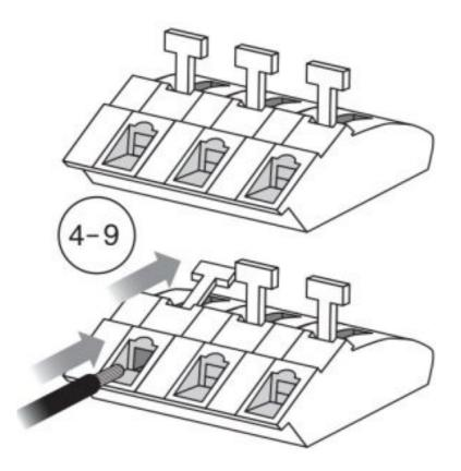
Use a screw driver to push the fastening clip over on the terminal block, place the cable into the terminal block and release the clip securing the cable.
