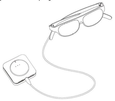
plug the USB-C cable of glasses into the computing unit
