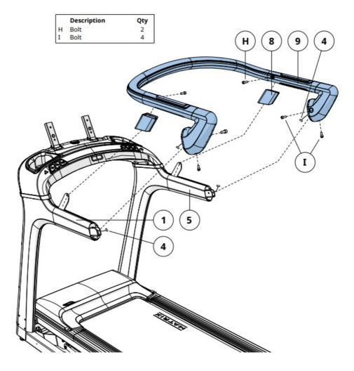
A Insert 4 HANDLEBAR CAPS (10) into HANDLEBAR (9).
