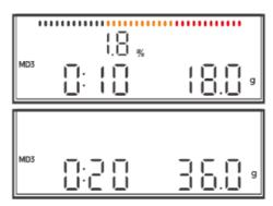
• After removing the cup or container, the scale will automatically start a countdown for reset after 10 seconds, allowing for continuous use.
