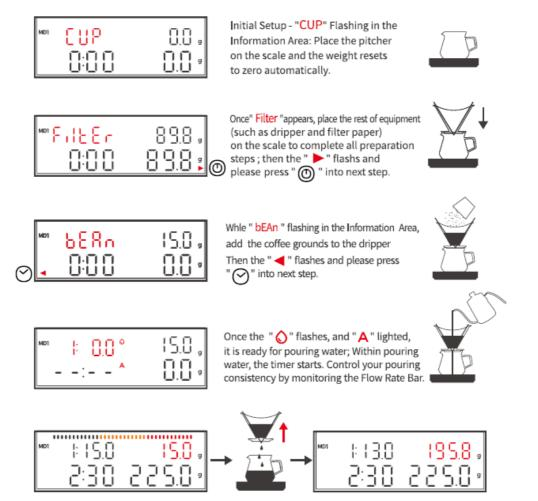
After finishing of water pouring, you can lift up the" Dripper" only in order to
