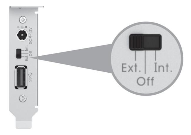
**OFF:** Turn off the USB port output power, when the external DAC and other products do not need USB bus power supply. In this mode, the devices such as USB flash disk which require USB bus power supply will not be available. **INT:** Internal power supply, USB bus power supply from SATA\_15P port on the end of card, the input power through the low noise LDO regulator and output from the USB port.
