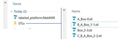
**Note** that the names of the saved STL files have been changed by adding the text from the applied labels to the part name as a prefix.
