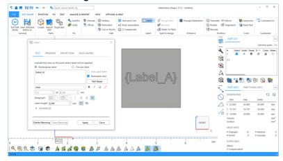
The "Auto Label" requires the label content to be applied in the form of a list to be able to provide the label planning of the part on the platform with the corresponding label content. The first entry in the list must correspond to the text template (without curly brackets!) of the label planning:
