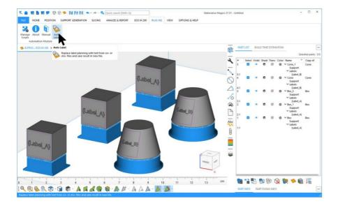
A dialog appears in which a profile can be selected, and parameters can be adjusted. Select the profile to be used and press the "**EXECUTE**" button to start automatic labeling.
