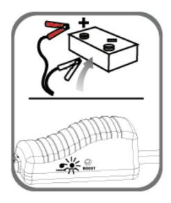
**RED LIGHT** on with buzzing -The connection is incorrect. The clamps are reverse of the correct set up. Refer to STEP 2 of the "Starting a Vehicle" instructions.
