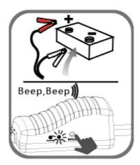
**No light and no buzzing** -The vehicle battery could be damaged or extremely low. Confirm the cables are properly connected. Press the BOOST button. When the light illuminates a steady green, start the vehicle within 30 seconds.
