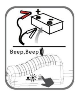
**GREEN LIGHT** blinking with buzzing -The vehicle battery is low. Press the BOOST button. When the light illuminates a steady green, start the vehicle within 30 seconds.
