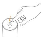
2. Press and hold the power button for 2 seconds until the blue light blinks.
