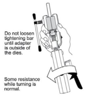
8. Grasp the yoke and rotate the tool Counter-clockwise to remove the adapter from
