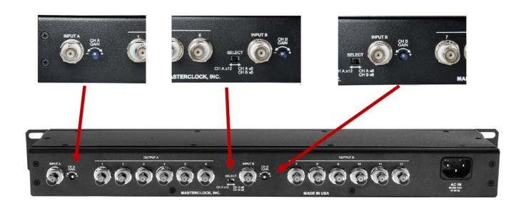
The Select switch will allow you to output channel A with a single input across all 12 outputs, or use channels A and B with their respective inputs and outputs independently.
