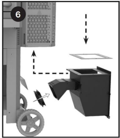
Replace hopper. Replace the gaskets Replace the fan. Reconnect wires.
