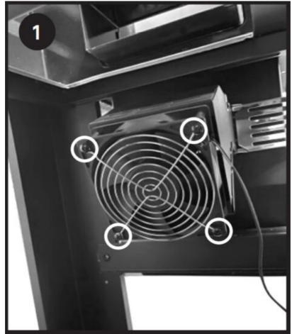
Remove the fan from the lower housing, you will reuse.
