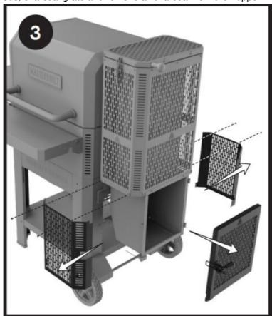
Remove the bottom hopper shroud and hopper door.
