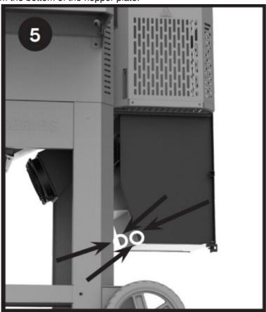
Remove the 2 screws and nuts from lower hopper mounting bracket.
