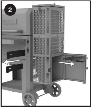
Remove the shutdown slides, charcoal grate and remove all charcoal from the hopper.
