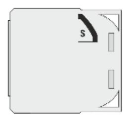
**WARNING:** Service button **S must NOT be used** when module is connected to 110-230V power supply. Durability of the device depends on applied load. For resistive load (light bulbs, etc.) and 4A current consumption of each individual electrical device, the durability exceeds 70.000 switches of each individual electrical device.
