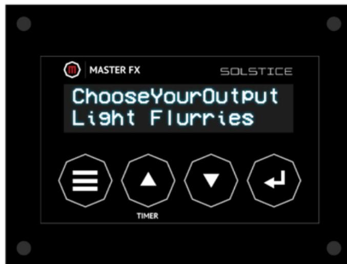
**SNOW OUTPUT SET:** When operating manually, you are able to change the density of snow, Choose between 1-100%. NOTE: When operating at a value over 50%, there is a risk of moisture accumulation. Avoid positioning the output nozzle over high traffic areas.
