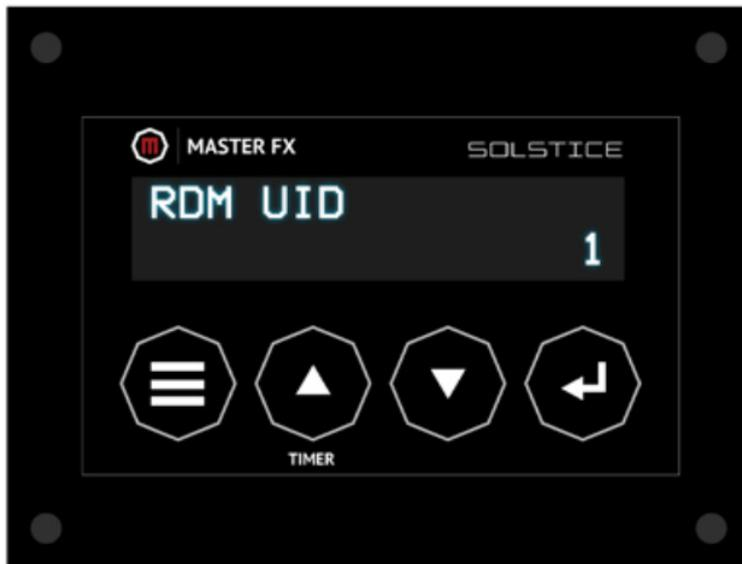
W-DMX: If you're operating via the optional wireless DMX, turn the power on for wireless DMX attachments by going through the settings and selecting "On."
