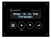
3. Before proceeding, it is important to understand what each button and setting does. Please see the diagram below for the button layout. To open settings, touch the menu button, scroll using the Up/Down arrows, and save your setting by pressing enter.
