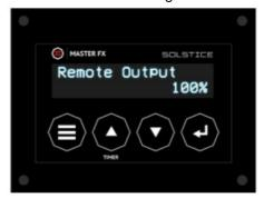
**PURGE MODE:** If your Solstice runs out of fluid, promptly refill the fluid tank and reconnect. Next, scroll through the settings to "Purge Mode". Press and hold the enter button to begin purging (the screen will read "On"). Hold the enter button until Snow comes out of the output nozzle. Release to stop the process.
