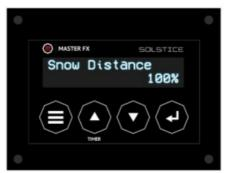
**TIMER:** You can operate your Solstice with an integrated timer by simply pressing the up arrow on the homescreen. To cancel the timer operation, select the enter button.
