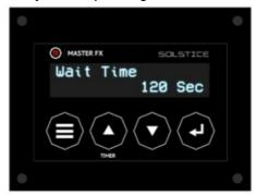
**RUN PREVIOUS SETTING:** When "On", the Solstice saves all operating settings for next use. **REMOTE OPERATION:** The Solstice can also be controlled by a wired remote. Once connected, the remote precedes all other operation modes except for DMX. To stop and start Snowing, use the power switch on the bottom of the remote. The snow output can be controlled using the **dial.**
