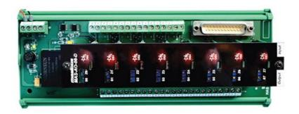
Masibus Analog Output Field Interface Board has 8 channels that accepts various types of current/voltage signals and converts them to isolated current/voltage signals. It is compact universal DIN rail mounted with labeled input and output connections. Independent zero & span adjustment for each channel is possible.
