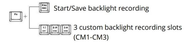
Press Fn+1 to choose CM1-slot then press FN+ESC to start backlight recording. Then choose the keys you want have lit.
