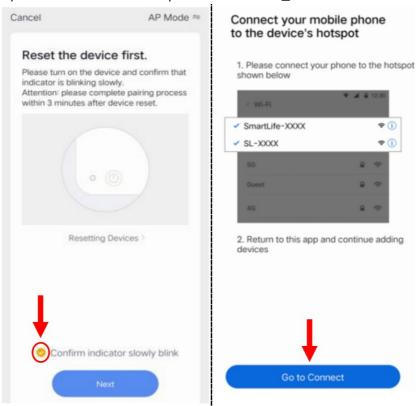
**Step 13:** After selecting a hotspot like "Smart Life\_xxxx" in the Wi-Fi setting page, go back to the App and it will connect automatically.
