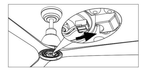
Install the diffusers as illustrated to finish the installation.
