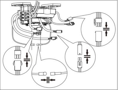
Carefully pull up and install the ceiling canopy as illustrated
