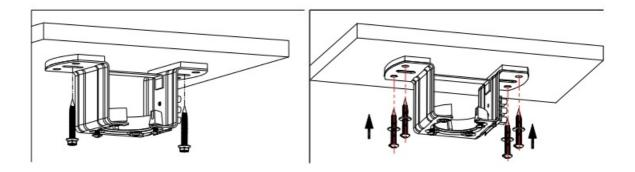
Secure the hanger bracket to ceiling beam or a suitable piece of timber inserted between the ceiling beams using the two long screws, or the four shorter screws supplied with the package.
