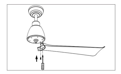
Install the blades to the bottom of the motor. Tighten and secure blade with screw and washer provided. Repeat
