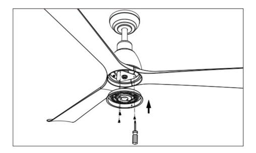
Install the LED light plate onto the steel bracket as illustrated with the 3 supplied screws. Connect LED with power by the quick connectors.
