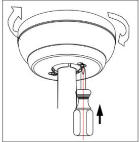
Carefully put the screw cap on using the piece of magnetic supplied.
