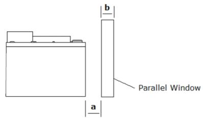
The front of the engine housing to the furthest surface of the window should not exceed a+b ( $a \le 0.1$ mm,  $b \le 2$ mm).
