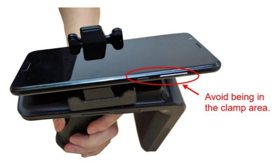
2. Pull one of the clamps to the side, meanwhile push the smartphone down until it is firmly secured.
