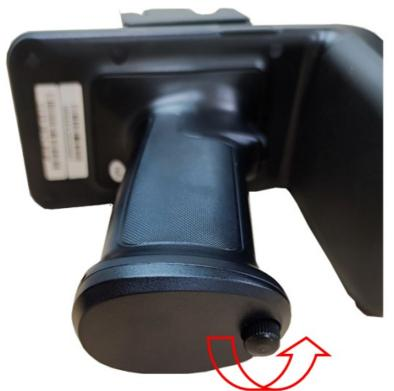
2. Open the cap at the bottom of the handle and remove the battery.
