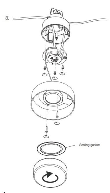
Use Ø2mm stainless steel cable (not included). Keep in mind the weight of each lamp when choosing the suspension system.
