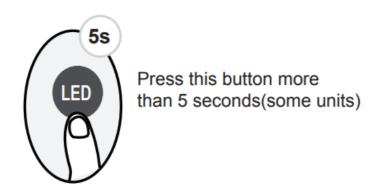
Keep pressing this button more than 5 seconds, the indoor unit will display the actual room temperature. Press more than 5 seconds again will revert back to display the setting temperature.
