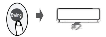
If continue to press the SWING button, five different airflow directions can be set. The louver can be move at a certain range each time you press the button. Press the button until the direction you prefer is reached.
