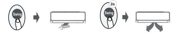
The horizontal louver will swing up and down automatically when pressing Swing button. Press again to make it stop.
