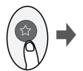
Push this button when remote controller is on, the system will automatically revert back to the previous settings including operating mode, setting temperature, fan speed level and sleep feature (if activated).
