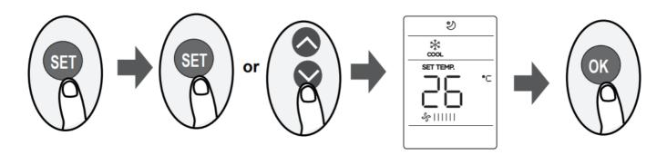
Press the SET button to enter the function setting, then press SET button or TEMP or TEMP button to select the desired function. The selected symbol will flash on the display area, press the OK button to confirm.
