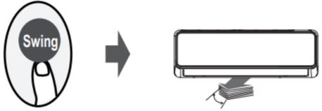
The horizontal louver will swing up and down automatically when pressing the Swing button. Press again to make it stop
