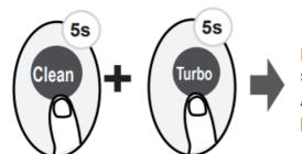
Press together **Clean** button and **Turbo** button at the same time more than 5 seconds to activate Lock function. All buttons will not response except pressing these two buttons for two seconds again to disable locking.
