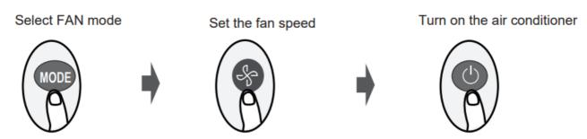
**NOTE:** In FAN mode, you can't set the temperature. As a result, no temperature displays in remote screen.
