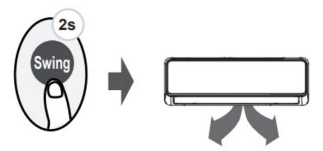
Keep pressing this button for more than 2 seconds, and the vertical louver swing function is activated. (For the units with vertical louver swing feature)
