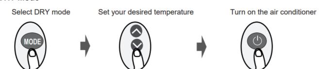
**NOTE:** In DRY mode, fan speed can not be set since it has already been automatically controlled.
