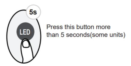
Keep pressing this button more than 5 seconds, the indoor unit will display the actual room temperature. Press more than 5 seconds again will revert back to display the setting temperature.
