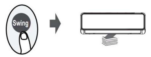
If continue to press the SWING button, five different airflow directions can be set. The louver can be moved within a certain range each time you press the button. Press the button until the direction you prefer is reached.
